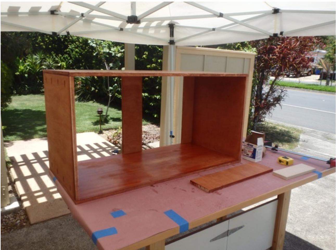
Good thing I did this, 'cause I quickly found out that I'd made the shelf unit side panels that go on top too long – misread my own plans when I transferred from the plans to the cut sheet. A couple of quick cuts solved the problem – sure better than looking for the board stretcher!
